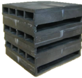
Figure 45: Isometric view of prototype heat exchanger [34]
