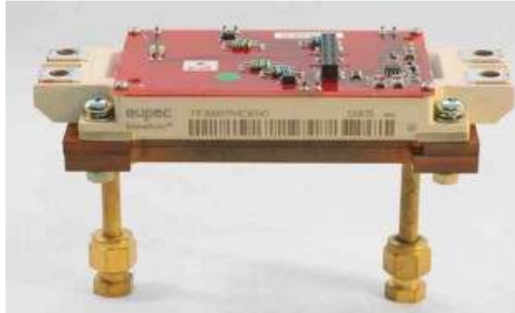
Figure 1.3 Integrated liquid cooled plate for IGBT module, Howes (2008)
