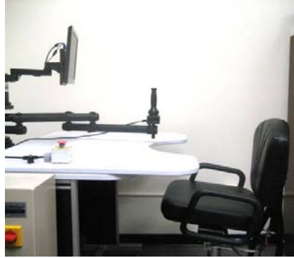
Figure 4.1: Set-up for Experiments 2 and 3. Participants were seated in a height-adjustable chair and were asked to execute arm movements while holding a robotic manipulandum that moves in two dimensions. The occluding board used in Experiment 2 is not shown.
