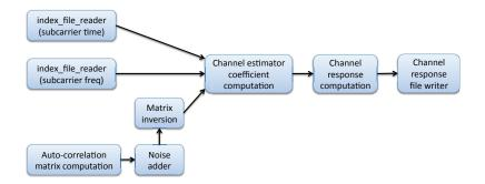
Figure 3: Dataflow graph for the wireless channel estimation example.
