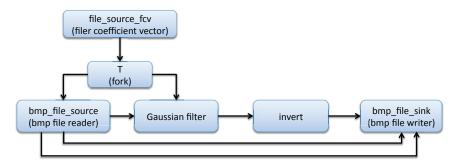
Figure 2: Dataflow graph for the Gaussian filtering example.
