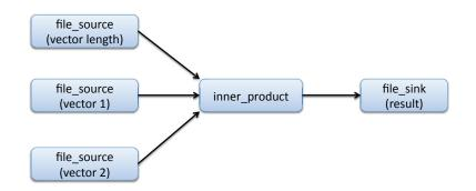
Figure 1: Dataflow graph for the inner product computation example.
