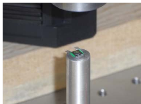
Figure 5-3. A device being rescanned after being assembled with the optical fibers.
