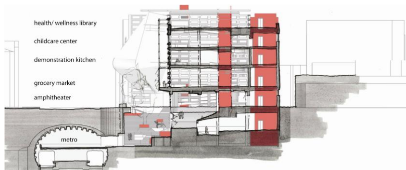
Figure 108: Cross Section at Metro and “Shaw Steps”
