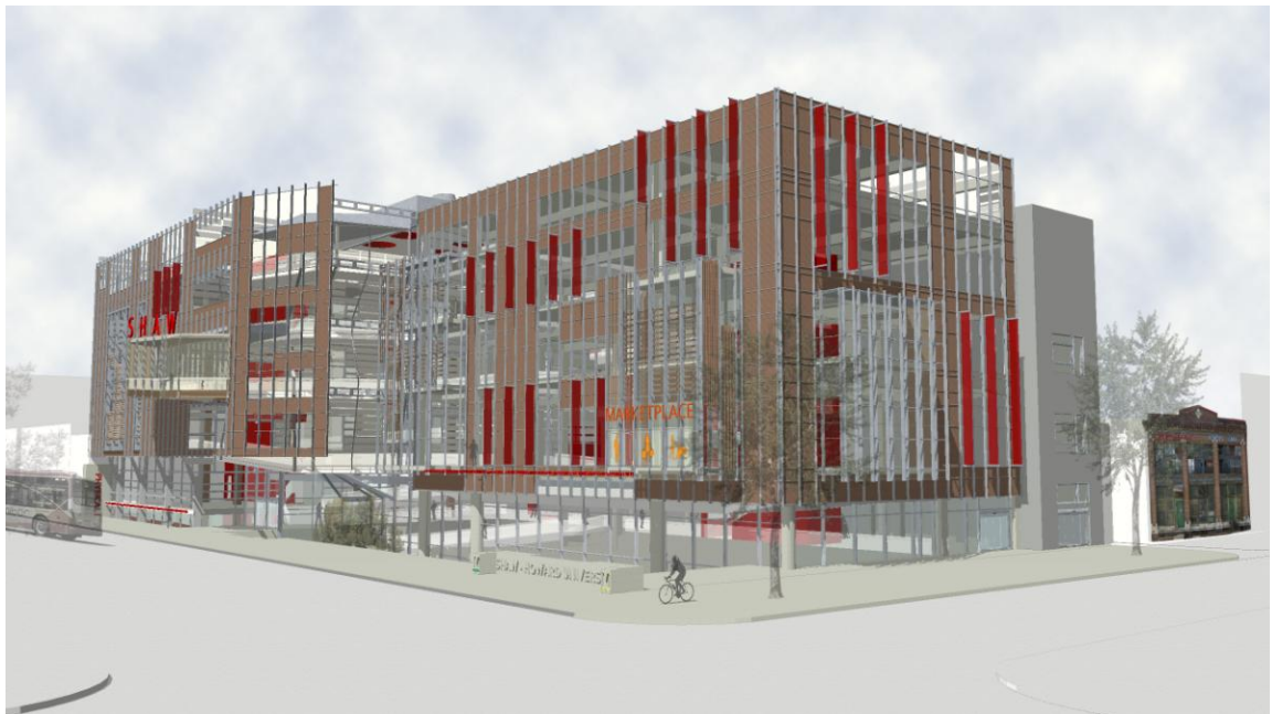
Figure 145: Façade Verticality Revisions. To Emphasis the vertical nature of the movement as well as break the building to the scale of the neighborhood and surrounding context, the horizontal members were reduced and scaled and the verticals were highlighted.
