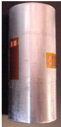
Figure 2.6: Cylindrical 2024 aluminum sample (2.54 cm in diameter) with axial and radial strain gages attached.
