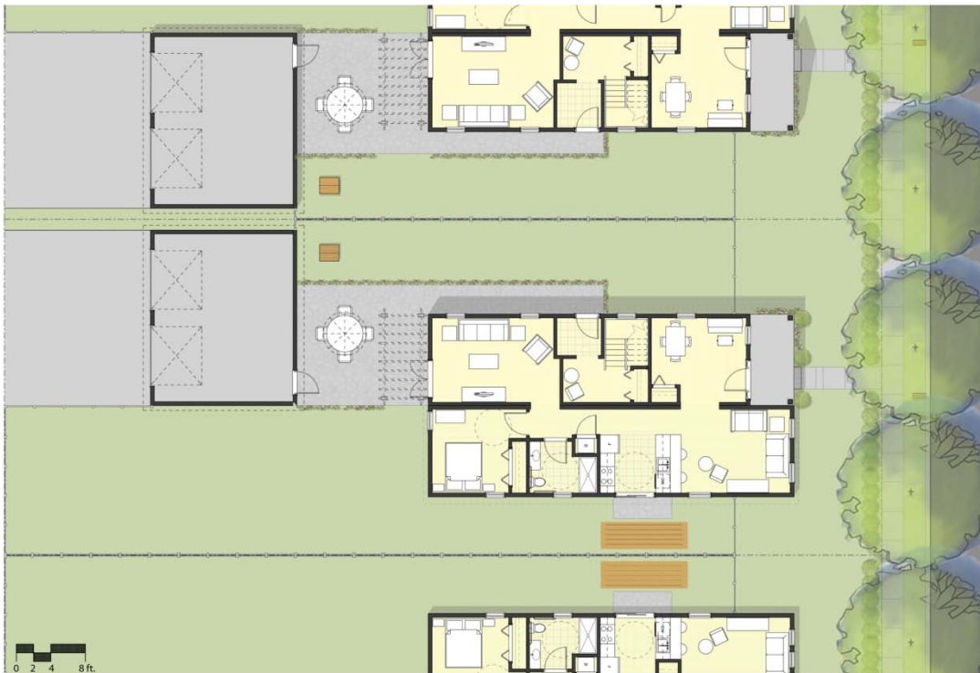
Figure 57: First and second floor plans the base component with two story expansion. Second story converted into a separate apartment.
