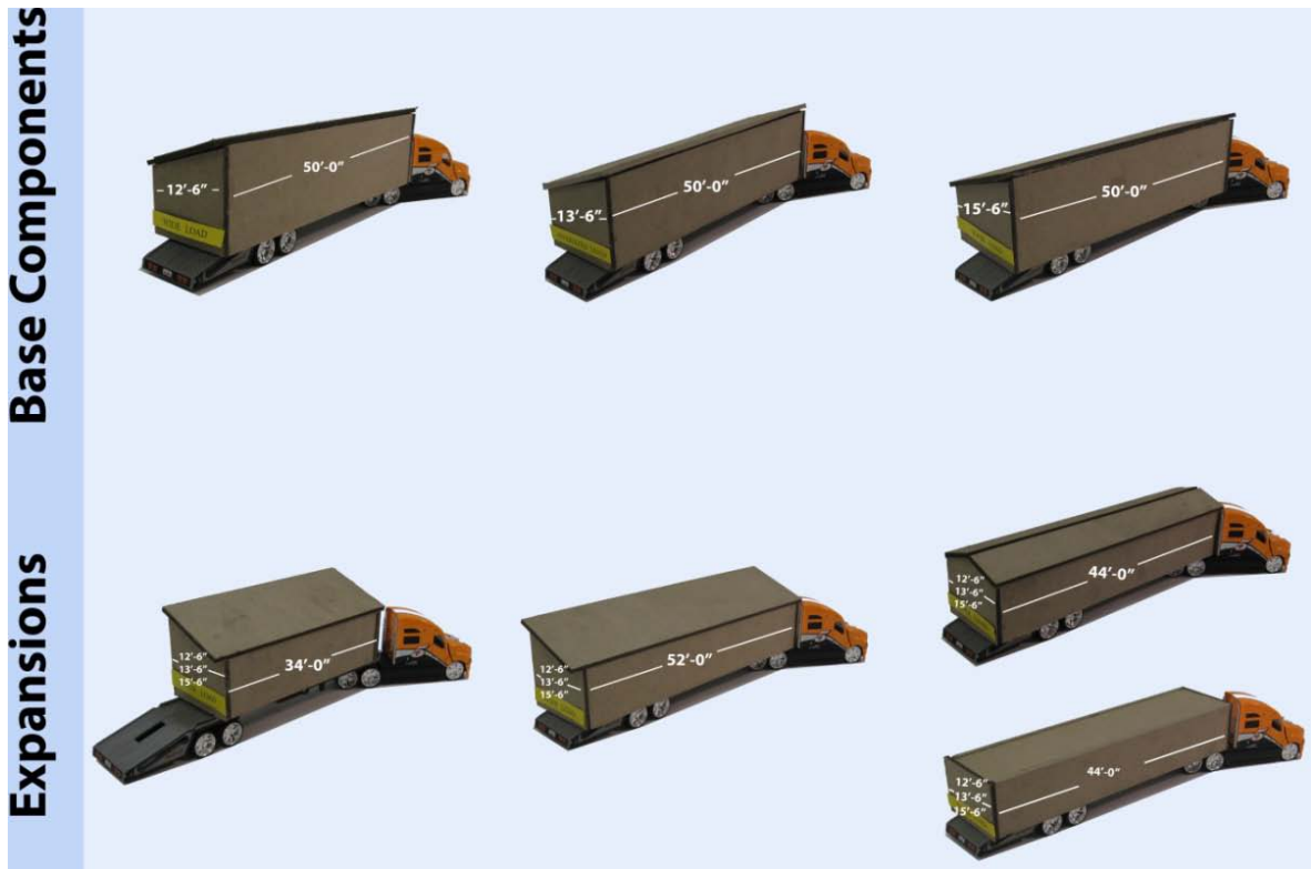
Figure 16: Transportation of Modules in 12'-6", 13'-6", and 15'-6"
