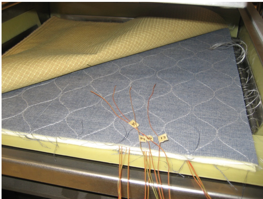
Figure 4.2 Thermocouples Against Top of Thermal Liner Prior to Placement
