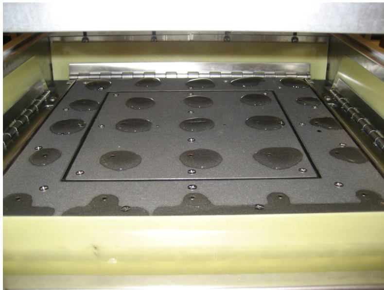
Figure 4.3: Moisture Entering Sweat Plate
