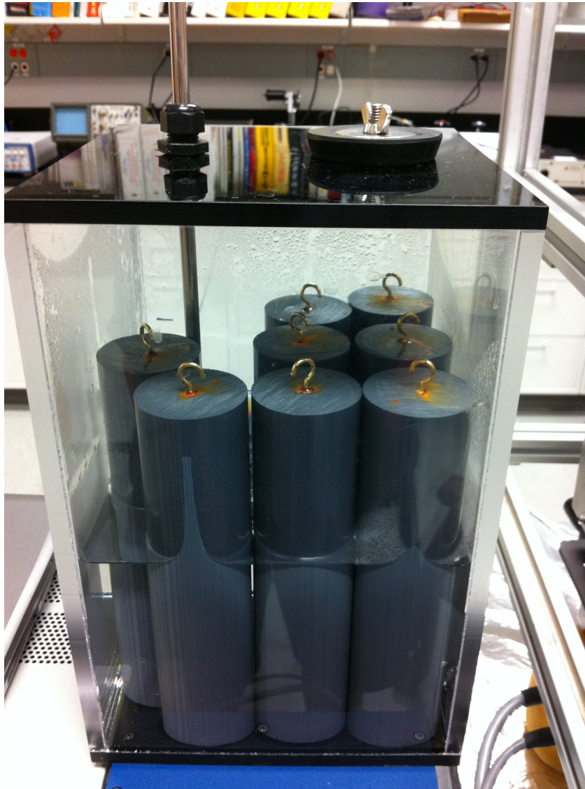
Figure 4.4: Water Reservoir With Solid Core PVC Pipe
