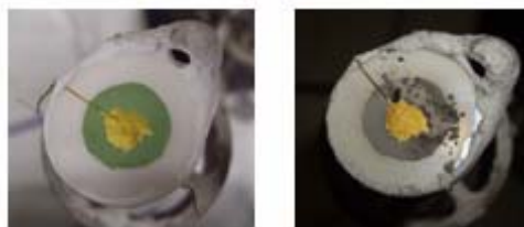
Figure VI.1. (Left) Picture of NiO/YSZ anode before operation under ethanol conditions. (Right) Picture of same anode after operation with ethanol. This SOFC was cooled down under reducing conditions (H 2 /Ar) leaving behind the partially delaminated Ni/YSZ anode.
