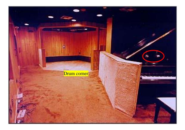
Illustration 4-3. Upper isolation room—piano, drums, and guitar. Note the placement of the microphones in the piano (circled).
