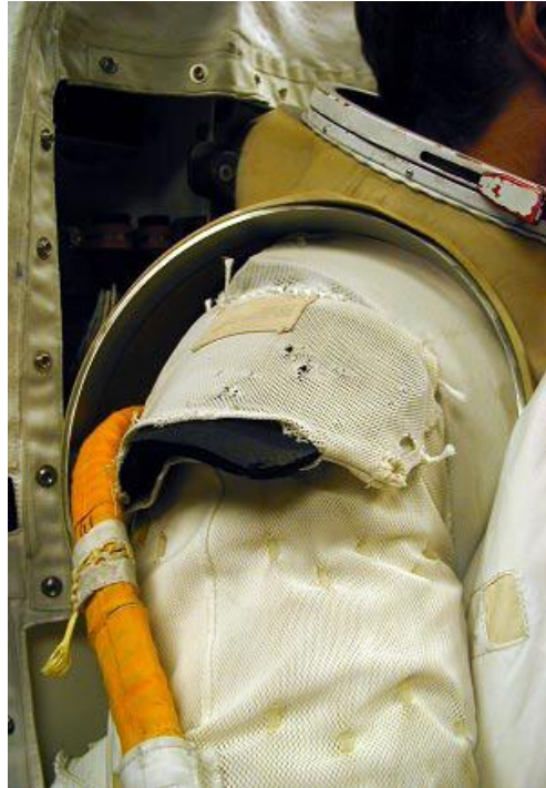
Figure 61. Side view of EMU HUT, example of clearance between scye bearing and shoulder. Image from [27].
