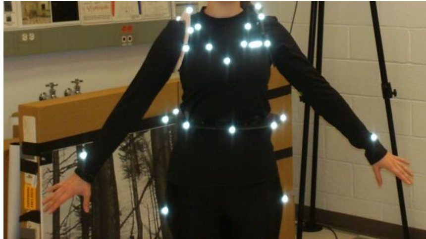
Figure 9. Subject wearing simulation suit: a spandex-like garment with simulated scye bearings and retro-reflective markers.
