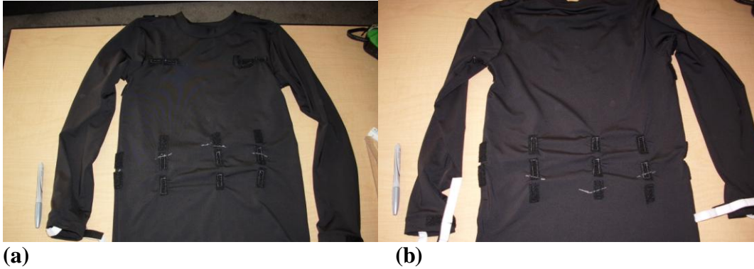
(a) (b) Figure 10. Front (a) and back (b) of the upper torso of the simulation suit, displaying Velcro points of attachment for simulated bearings.
