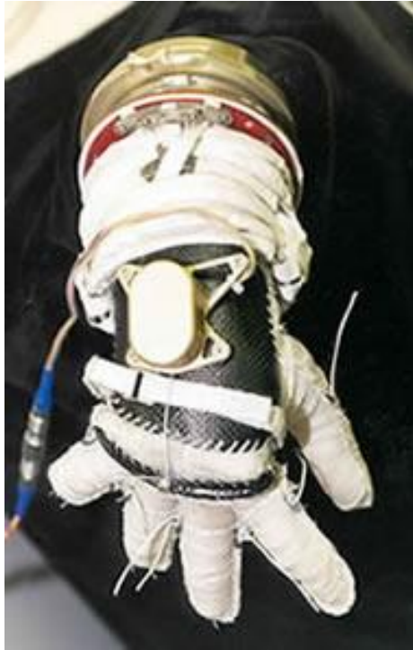
Figure 5. Power-assisted spacesuit glove design [12].
