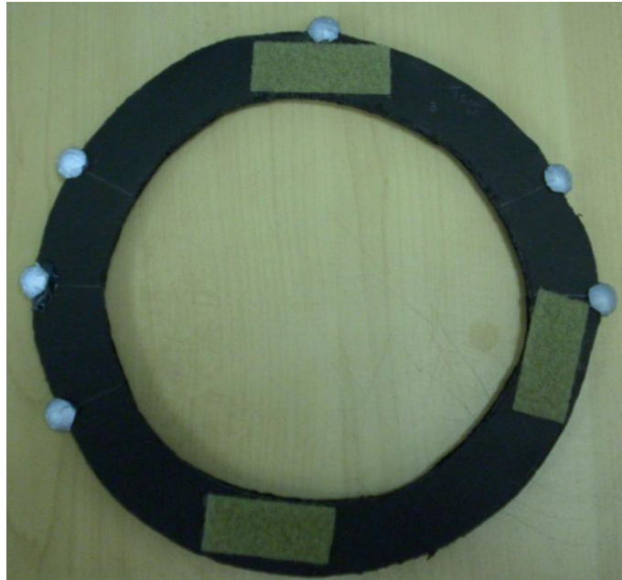
Figure 14. Example of foamcore scye bearing simulator with retro-reflective markers attached.
