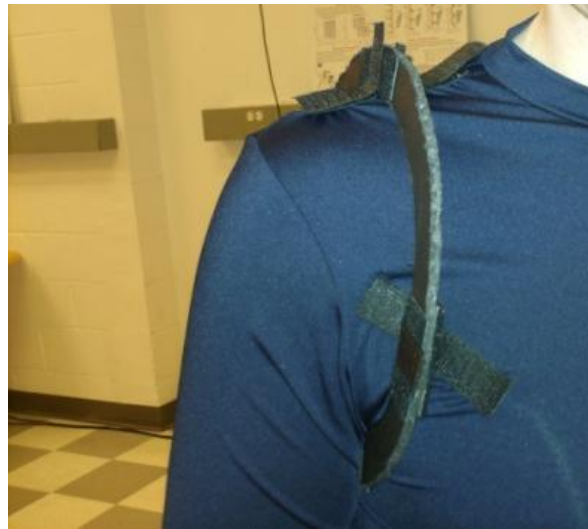
Figure 11. Image showing two of three attachment points of the scye bearing. The three points of attachment for the bearing are: top of the shoulder, chest, and underarm (not visible).
