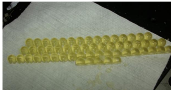
Figure 17. A set of scye bearing markers produced using a rapid prototyping machine.
