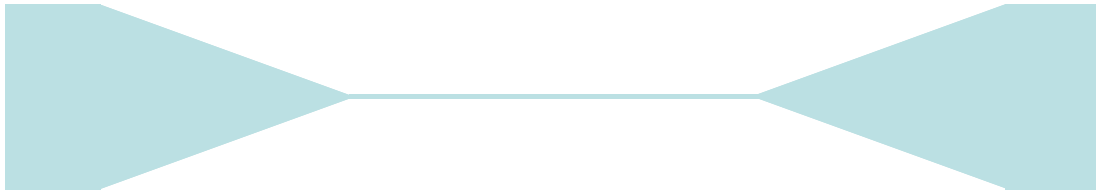
Figure 10.1 – Creation of heater by removing all unwanted metal.
