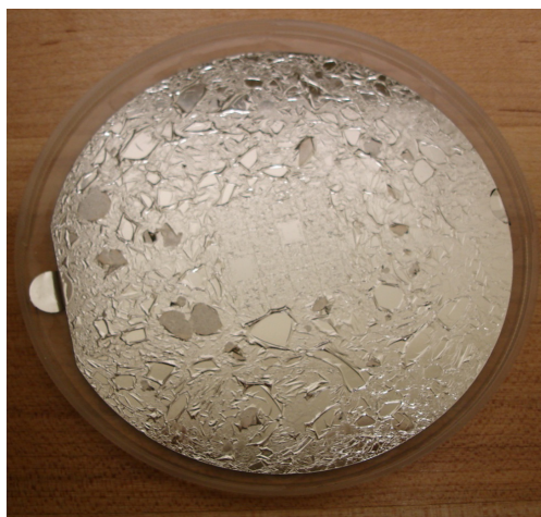
Figure 5.6 – Overheated photoresist causes adhesion problems for the metal.
