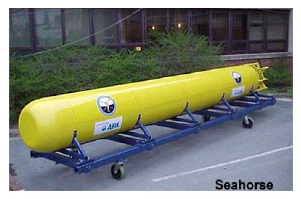
Figure 1-8: US Navy Seahorse UUV, designed at Penn State ARL.
