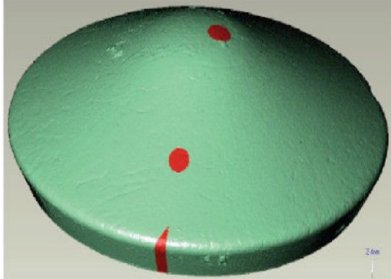
Figure 3.93. The near stagnation and flank core points, along with a shoulder point, indicated in red on the Stardust Return Capsule. 84
