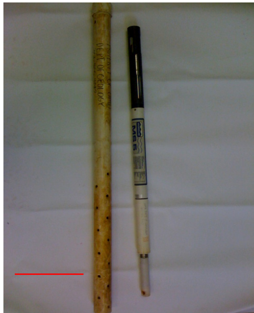
Figure 6: Pictured is the Hach Hydrolab MS5 field probe used at the Green Castle, Cherry Hill and Downstream Cherry Hill site. The probe is secured inside a PVC pipe to protect the sensors during periods of high flow. The scale bar shows 1 ft.
