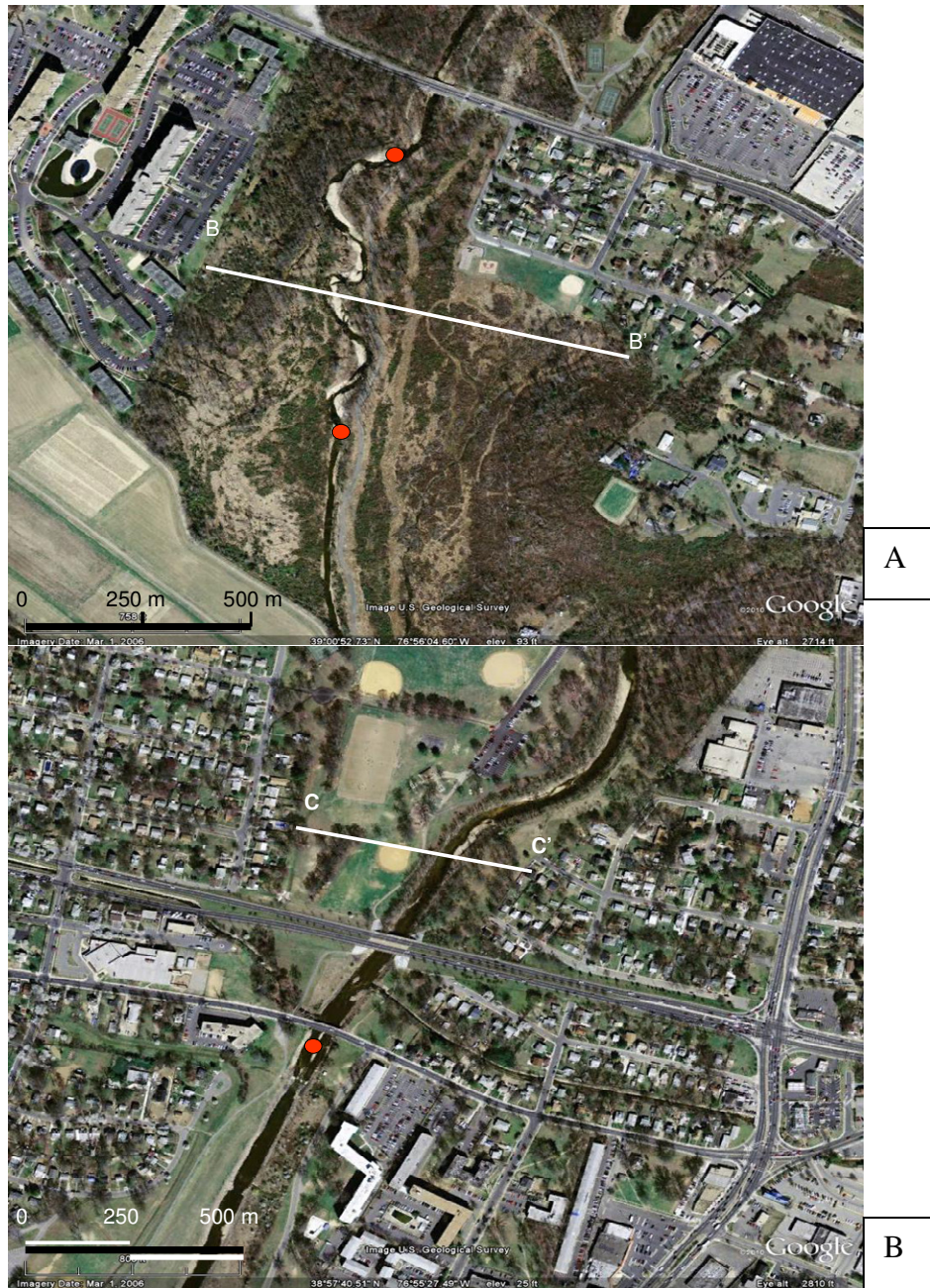
Figure 28: (A) Cherry Hill upstream and downstream site (marked with red circles). Note the extensive floodplain remnant left intact. (B) Lower NE Branch watershed (USGS NE Branch gauge marked with red circle). Note the channelization in B where storm sewer systems are routed directly to the channel.
