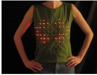
Figure 87. Electronic Clothing Hybrids: LED shirt [12]
