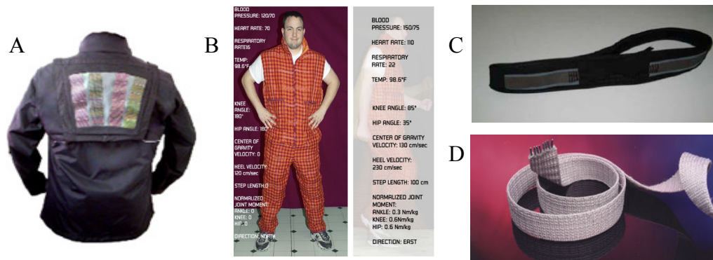
Figure 2. E-textiles and smart fabrics major development motivators: a. Civilian (Solar Jacket)[16], b. Research (Hookie suit)[17], c. Medical (Chest strap)[18], d. Military (Fabrics information cable.)[14]
