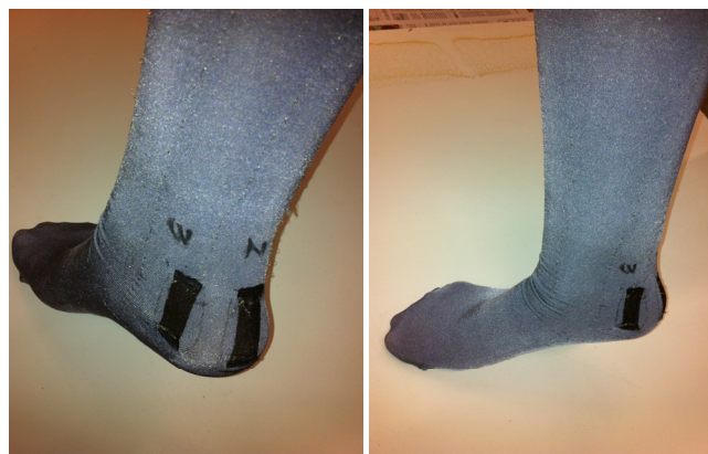
Figure 79. PI-coated fabric sensors on sock
