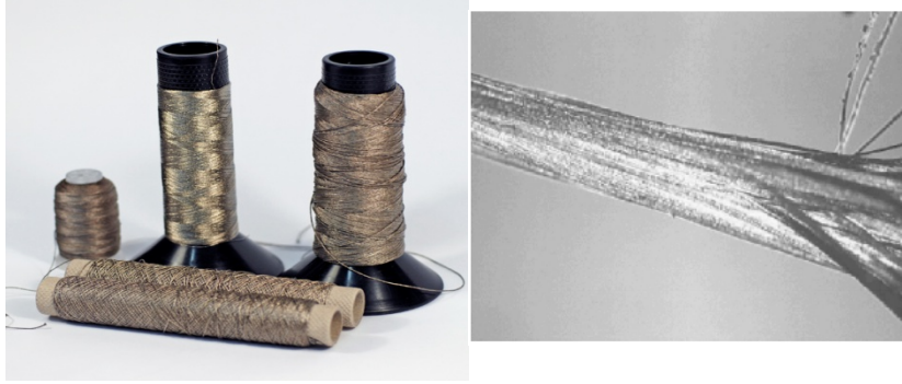
Figure 102. a. Conductive thread-silver plated nylon and b. 100% stainless steel fiber bundle [78]
