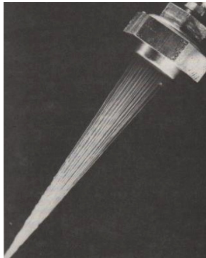
Figure 137. Solution emerging from spinnerette to form filament yarn [113]
