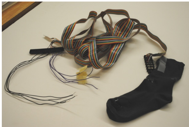
Figure 77. Acquisition setup for sensorized sock.
