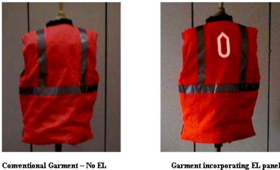
Figure 93. Canesis Electroluminescent (EL) safety garment: a. Garment with EL display off, b. with display on [68].
