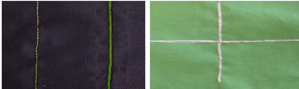
Figure 108. a. Exposed and insulated thread by couching and b. insulated thread by fabric paint [12]
