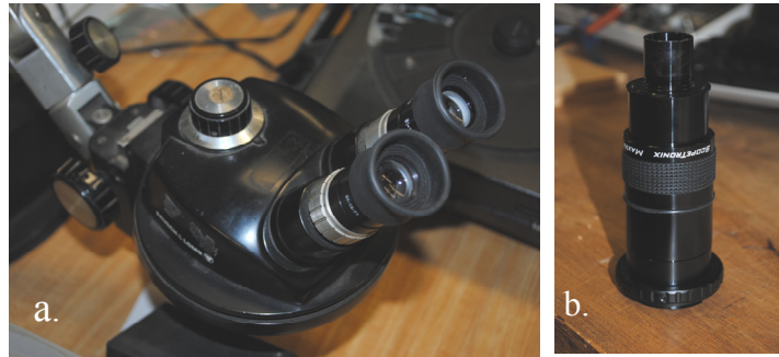
Figure 56. Optical microscope used for viewing the textures of the different fabrics: a. ocular and diopter, b. camera adaptor
