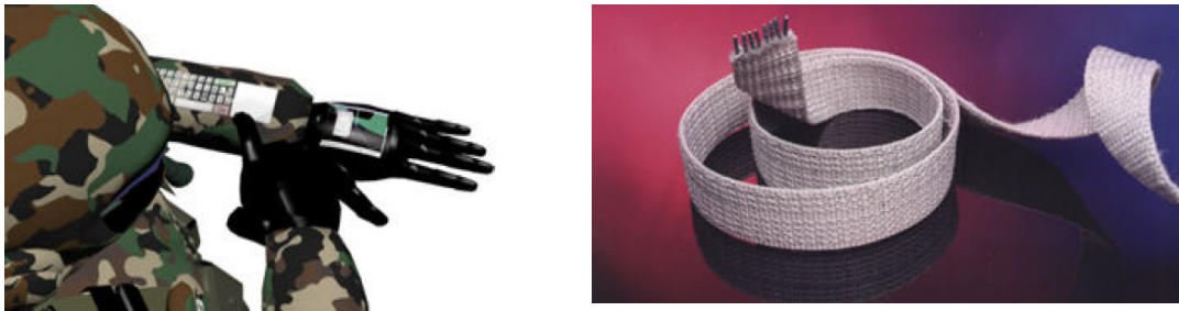
Figure 100. E-textiles applications in defense: a. Soldier portable computer [14], b. textile information cable .
