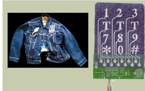
MIDI Jacket with capacitive fabric keyboard
