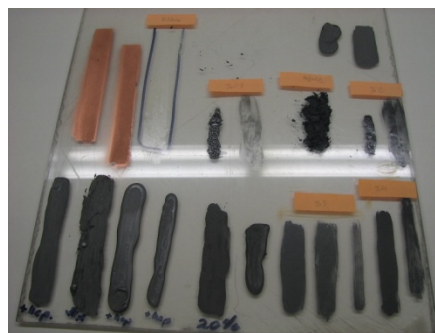
Figure 14. Acrylic board with raw materials to be tested for their conductive properties.
