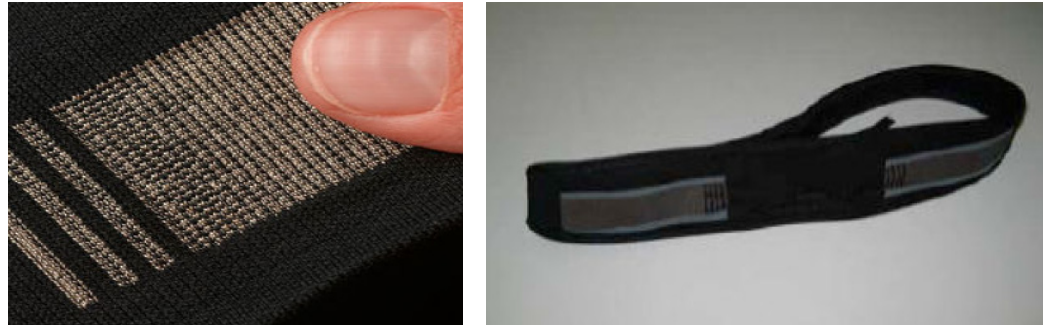
Figure 95. Textronics conductive elastic fabric used for ECG chest straps [15]: a. Close up of fabric sensor, b. Chest strap.
