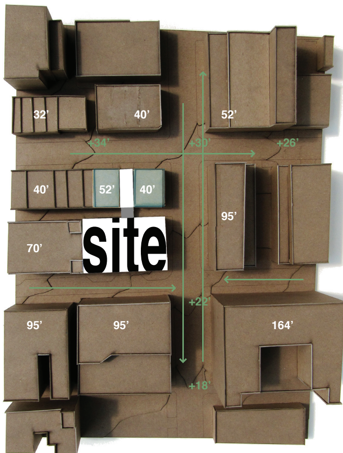
Figure 21_ Site massing model showing context bulk and mass, slope, and traffic movement around the site.
