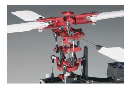
Figure 3.36: Rotor Assembly of an RC Helicopter including Swash plate
