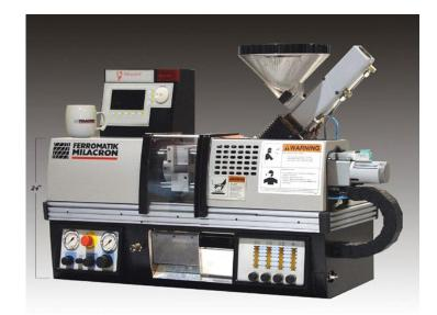
Figure 1.2 Babyplast<sup>®</sup> injection molding machine
