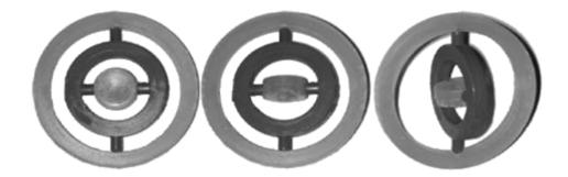
Figure 2.5 2-DOF movement of in-mold assembled gimbal [89]
