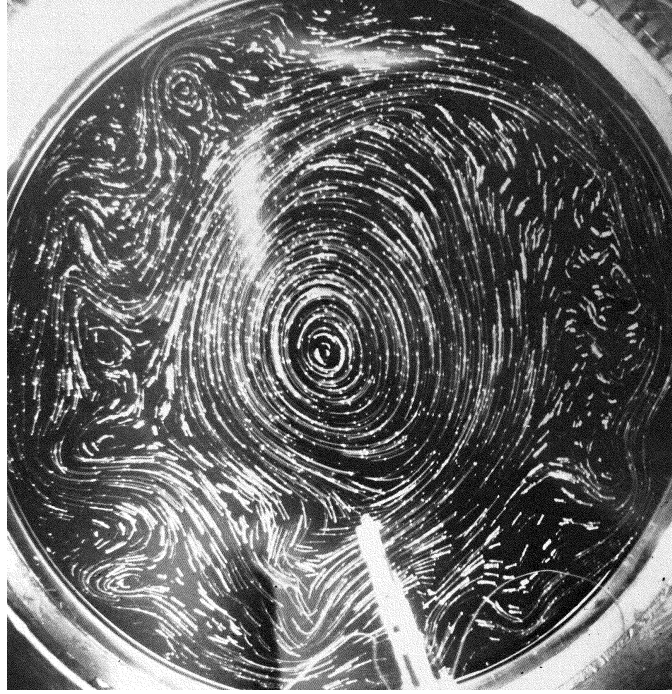
Figure 3.9: Classical convection in a rotating cylinder by [53]. In this image, the vessel is heated at the rim and cooled at the center, driving convection.
