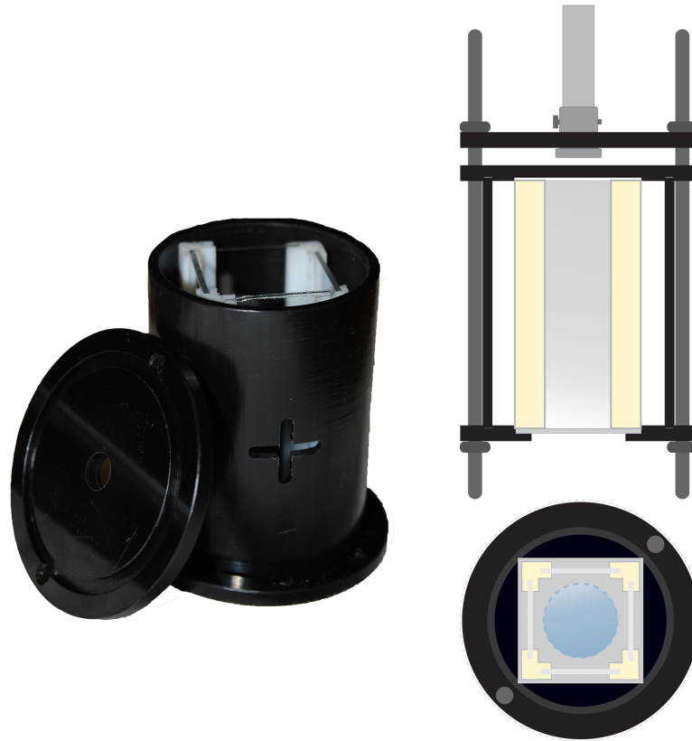
Figure 2.4: Image and diagram of the isolation cell
