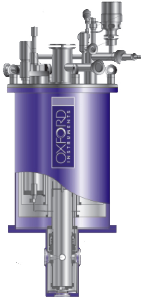
Figure 2.1: Cutaway of the Oxford Instruments OptistatSXM used in these experiments. The bulk of the cryostat is a liquid helium reservoir, while the central cylinder is the main testing space for the experiments. A vacuum chamber thermally insulates the entire unit. Image acquired from Oxford Instruments.
