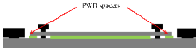
Figure 51: Use of PWB spacers can reduce beam bending in the top clamp.
