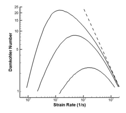
Figure 5.2: Damköhler number versus strain rate  $\alpha$  (log-log plot). Top dashed line: adiabatic flame. Three lower solid lines: sooting and radiating flames with  $Y_{soot,R} = 0$ (top), 1% (middle), 5% (bottom). The critical values of at the extinction limits are close to 1.
