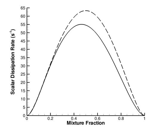
Figure B.2: Comparison between AEA and DNS scalar dissipation rates, with  $\chi_{st} = 6 \text{ s}^{-1}$ , and the matching condition for the mixture fraction  $Z_{st,+} = 0.15$ . Solid lines denote DNS data, while dashed lines denote AEA data.
