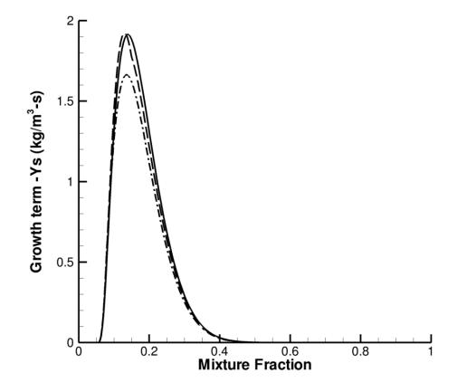
Figure B.11: Comparison between AEA and DNS soot growth terms appearing in Equation (2.16), with  $\chi_{st} = 6 \text{ s}^{-1}$ . Solid lines denote DNS data, dash-dotted lines denote AEA data with the matching condition for the mixture fraction specified as  $Z_{st,+} = 0.08$ , and dashed lines denote AEA data with  $Z_{st,+} = 0.15$ .
