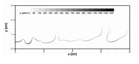
(a) Flame heat release rate  $[MW/m^3]$
