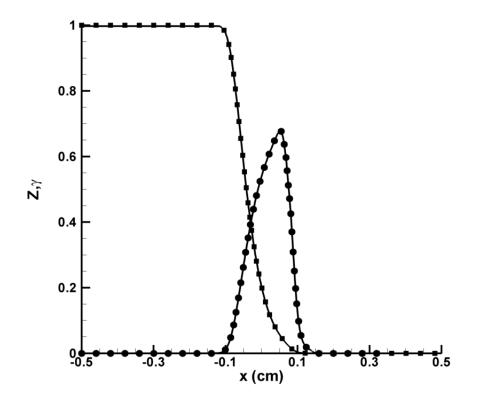
Figure A.2: Spatial variations of mixture fraction Z (squares) and spray vapor mass fraction  $\gamma$  (circles) along the flame normal direction. Values of  $\gamma$  are multiplied by a factor 10 to facilitate the graphical display.
