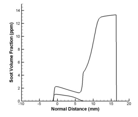
Figure 5.5: Soot volume fraction versus normal distance to the flame,  $\alpha = 20s^{-1}$ . Bottom line: flame with  $Y_{soot,R} = 0$ ; top line: soot-loaded flame with  $Y_{soot,R} = 2\%$ . Soot addition occurs at  $x \approx 17$  mm.
