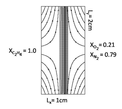
Figure 7.1: Computational configuration. Solid lines with arrows denote potential flow streamlines. Dotted lines represent temperature contours. Solid black line within the temperature contours indicates the stoichiometric mixture fraction identifying the flame location.
