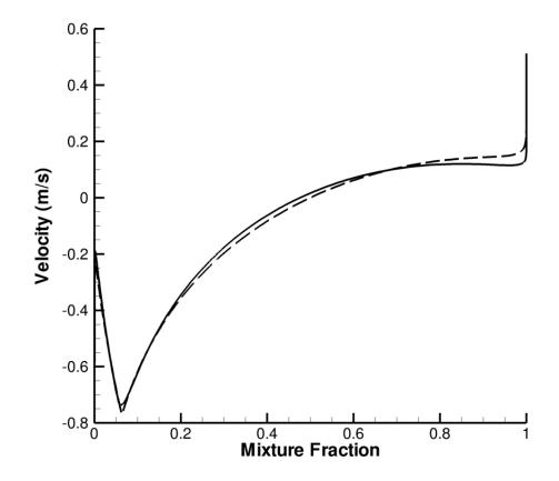
Figure B.3: Comparison between AEA and DNS *x*-direction velocities, with  $\chi_{st} = 6 \text{ s}^{-1}$ , and the matching condition for the mixture fraction  $Z_{st,+} = 0.15$ . Solid lines denote DNS data, while dashed lines denote AEA data.
