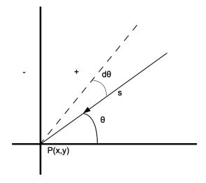
Figure 3.2: Schematic of domain and setup to calculate radiation absorption by integrating RTE. The left and right of the point under consideration P(x, y) are denoted by '-' and '+' respectively.
