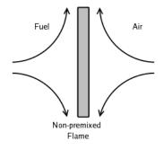
Figure 1.1: Schematic of a non-premixed flame
