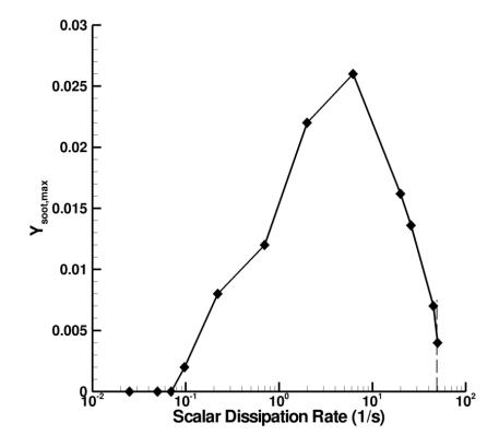
Figure 4.5: Laminar flamelet database (4). Peak soot mass fractions versus fuel-air mixing rate, corresponding to the maximum soot mass fraction in the domain. Vertical dashed lines mark the lower and upper limits of the flammable domain,  $\chi_{st}^{LL}$  and  $\chi_{st}^{UL}$ .
