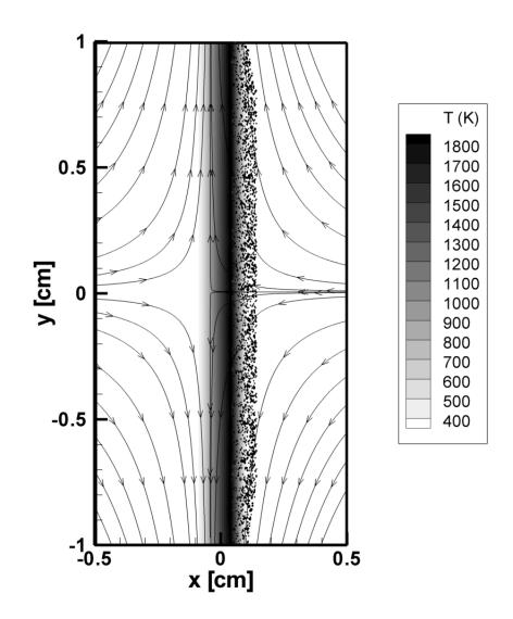
Figure A.1: Laminar counterflow diffusion flame (ethylene is injected at x = -0.5 cm; air is injected at x = 0.5 cm). The plot shows selected flow streamlines and temperature iso-contours. The black dots at  $0 \le x \le 0.145$  cm mark the location of the liquid water droplets.
