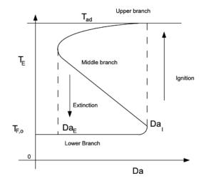
Figure 1.2: S-curve. Schematic illustration of the dependence of the maximum flame temperature on the Damköhler number.
