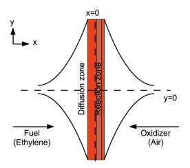
Figure 3.1: Schematic of counterflow flame. The flame (shaded brown) is located to the right of the stagnation flame (dashed lines). The reaction zone is embedded in a much thicker diffusion zone (shaded red)
