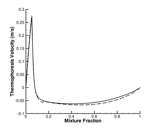
Figure B.4: Comparison between AEA and DNS *x*-direction thermophoretic velocities, with  $\chi_{st} = 6 \text{ s}^{-1}$ , and the matching condition for the mixture fraction  $Z_{st,+} = 0.15$ . Solid lines denote DNS data, while dashed lines denote AEA data.
