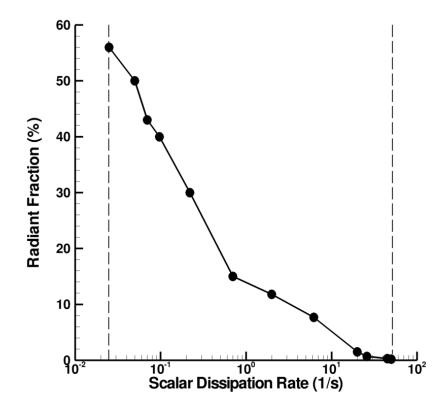
Figure 4.4: Laminar flamelet database (4). Radiant fraction (ratio of radiation cooling rate to flame heat release rate, with both quantities integrated across flame zone) versus fuel-air mixing rate. Vertical dashed lines mark the lower and upper limits of the flammable domain,  $\chi_{st}^{LL}$  and  $\chi_{st}^{UL}$ .
