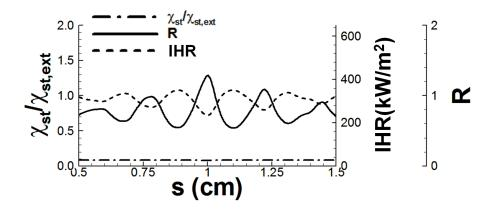
Figure 7.4: Spatial distribution of normalized scalar dissipation rate, integrated heat release rate and the weakness factor along the flame surface for Case B at t = 5.9ms.
