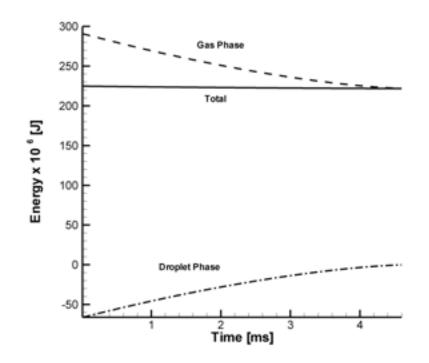
Figure C.6: Conservation of energy (droplet diameter 20  $\mu$ m). The solid black curve is the total energy of the system, expressed as the sum of gas phase (dashed lines) and liquid phase (dash-dotted lines) energies. The total energy of the system remains nearly constant, showing a variation of only 1% over the course of the droplet's lifetime (4.5 ms).
