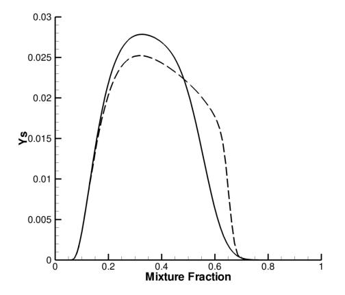
Figure B.6: Comparison between AEA and DNS soot mass fractions, with  $\chi_{st} = 6 \text{ s}^{-1}$ , and the matching condition for the mixture fraction  $Z_{st,+} = 0.15$ . Solid lines denote DNS data, while dashed lines denote AEA data.
