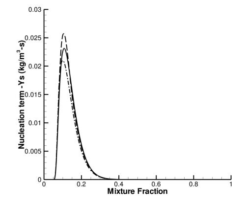
Figure B.10: Comparison between AEA and DNS soot nucleation terms appearing in Equation (2.16), with  $\chi_{st} = 6 \text{ s}^{-1}$ . Solid lines denote DNS data, dash-dotted lines denote AEA data with the matching condition for the mixture condition specified as  $Z_{st,+} = 0.08$ , and dashed lines denote AEA data with  $Z_{st,+} = 0.15$ .
