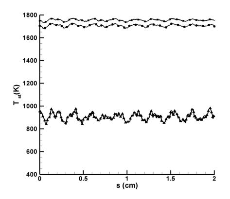
Figure A.4: Temperature variations as a function of arc length s measured along the stoichiometric contour. The lower (upper) curve corresponds to methodology M1 (M2); the middle curve corresponds to the methodology due to Bilger, see Equation (A.12).
