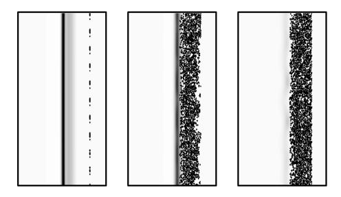
Figure 7.2: Heat release rate isocontours with spray overlay (small dots) for Case B at t = 0.3, 5.7, 6.2 ms (going from left to right as the simulation progresses).
