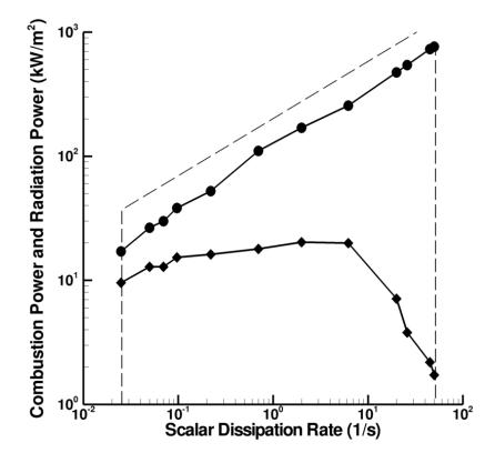
Figure 4.2: Laminar flamelet database (4). Combustion heat release rate  $\dot{q}_c''$  (circles) and flame radiative power  $\dot{q}_r''$  (diamonds) versus fuelair mixing rate  $\chi_{st}$ . The top dashed line shows a reference square root variation; vertical dashed lines mark the lower and upper limits of the flammable domain,  $\chi_{st}^{LL}$  and  $\chi_{st}^{UL}$ .
