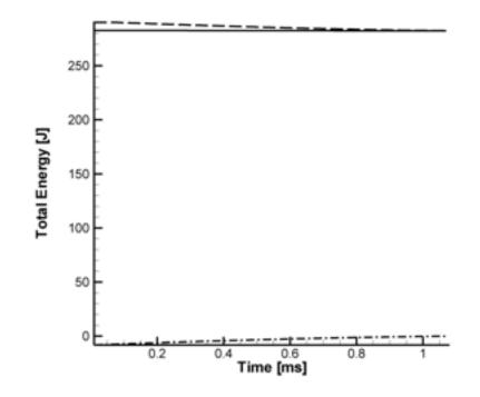
Figure C.2: Conservation of energy (droplet diameter  $10\mu$ m). The solid black curve is the total energy of the system, expressed as the sum of gas phase (dashed lines) and liquid phase (dashdotted lines) energies. The total energy of the system remains nearly constant, showing a variation of only 0.1% over the course of the droplet's lifetime (1 ms).
