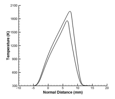
Figure 5.4: Temperature versus normal distance to the flame,  $\alpha = 20s^{-1}$ . Top line: flame with  $Y_{soot,R} = 0$ ; bottom line: soot-loaded flame with  $Y_{soot,R} = 2\%$ .  $x \leq 5$  mm corresponds to the fuel (air) side of the flame.
