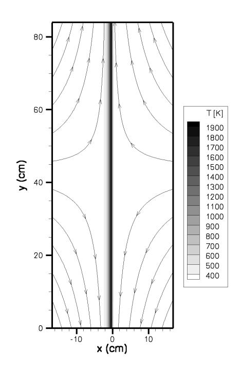
Figure 4.1: Laminar flamelet database. Fuel (ethylene) and oxidizer (atmospheric-air) are injected from the left and right respectively. The plot shows selected flow streamlines and temperature isocontours. In this case,  $\chi_{st} = 0.2 \text{ s}^{-1}$  and  $(L_x, L_y) = (33.6 \text{ cm}, 84 \text{ cm})$ .
