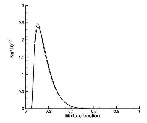
Figure B.5: Comparison between AEA and DNS soot number density, with  $\chi_{st} = 6 \text{ s}^{-1}$ , and the matching condition for the mixture fraction  $Z_{st,+} = 0.15$ . Solid lines denote DNS data, while dashed lines denote AEA data.
