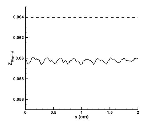
Figure A.5: Mixture fraction variations as a function of arc length s measured along the stoichiometric contour. The lower curve corresponds to the methodology of Bilger, see Equation (A.14); the upper curve corresponds to methodology M2.
