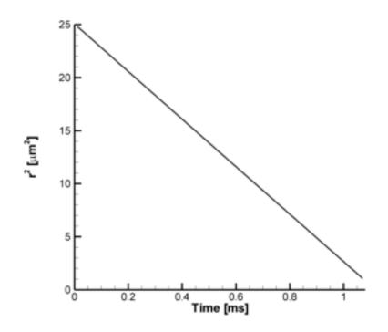
Figure C.3: The  $d^2$  law (droplet diameter 10  $\mu$ m). The square of the droplet's radius is plotted over time. The variation is linear, thus showing that the  $d^2$  law is satisfied for the evaporating droplet.
