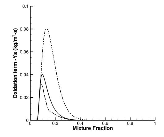
Figure B.8: Comparison between AEA and DNS soot oxidation terms, with  $\chi_{st} = 6 \text{ s}^{-1}$ . Solid lines denote DNS data, dash-dotted lines denote AEA data with the matching condition for the mixture fraction specified as  $Z_{st,+} = 0.08$ , and dashed lines denote AEA data with  $Z_{st,+} = 0.15$ .
