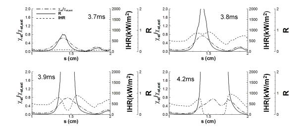
Figure 7.8: Distribution of the normalized scalar dissipation rate, integrated heat release rate  $(kW/m^2)$  and the weakness factor for the turbulent flames with spray at the four different times shown in Figure 7.7. The range of flame length shown here corresponds to that in Figure 7.6.
