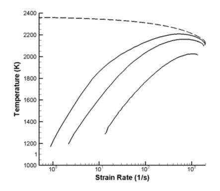
Figure 5.1: Peak flame temperature versus strain rate  $\alpha$  (log-linear plot). Top dashed line: adiabatic flame. Three lower solid lines: sooting and radiating flames with  $Y_{soot,R} = 0$ (top), 1% (middle), 5% (bottom). The end points of each solid line mark the lower and upper limits of the flammable domain.
