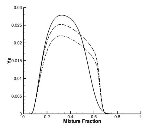
Figure B.9: Comparison between AEA and DNS soot mass fractions, with  $\chi_{st} = 6 \text{ s}^{-1}$ . Solid lines denote DNS data, dash-dotted lines denote AEA data with the matching condition for the mixture fraction specified as  $Z_{st,+} = 0.08$ , and dashed lines denote AEA data with  $Z_{st,+} = 0.15$
