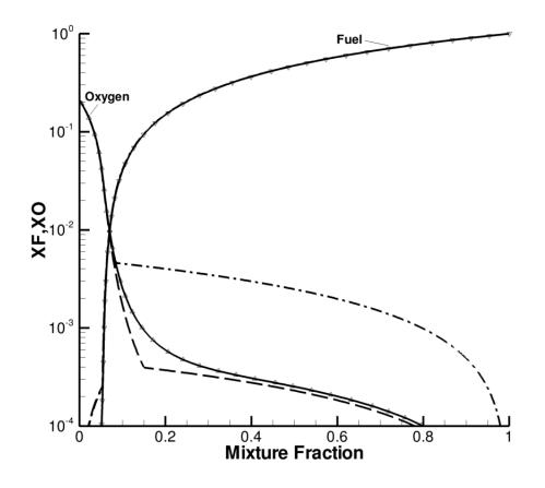
Figure B.7: Comparison between AEA and DNS fuel and oxidizer mole fractions, with  $\chi_{st} = 6 \text{ s}^{-1}$ . Solid lines denote DNS data, dash-dotted lines denote AEA data with the matching condition for the mixture condition specified as  $Z_{st,+} = 0.08$ , and dashed lines denote AEA data with  $Z_{st,+} = 0.15$ .
