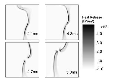
Figure 7.5: Temporal evolution of heat release rate isocontours for turbulent flame simulation without spray. These pictures are zoomed into a  $0.8 \text{ cm} \times 0.8 \text{ cm}$  region in which the flame undergoes a flame extinction event.
