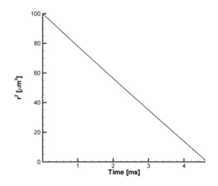
Figure C.7: The  $d^2$  law (droplet diameter 20  $\mu$ m). The square of the droplet's radius is plotted over time. The variation is linear, thus showing that the  $d^2$  law is satisfied for the evaporating droplet.
