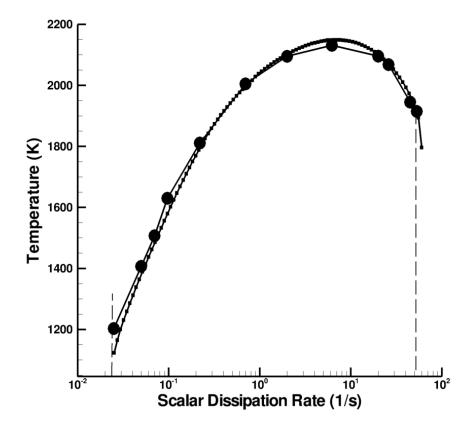
Figure 4.3: Laminar flamelet database (4, and equivalent AEA flame 3). Flame temperature [K] versus fuel-air mixing rate  $\chi_{st}$ . Circular symbols represent DNS data, while diamond shaped symbols represent the AEA data. Vertical dashed lines mark the lower and upper limits of the flammable domain,  $\chi_{st}^{LL}$  and  $\chi_{st}^{UL}$ .
