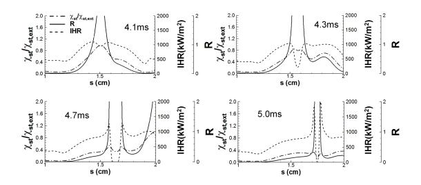
Figure 7.6: Distribution of the normalized scalar dissipation rate, integrated heat release rate  $(kW/m^2)$  and the weakness factor for the turbulent flames without spray at the four different times shown in Figure 7.5. Only part of the flame region near the location of extinction is shown here.
