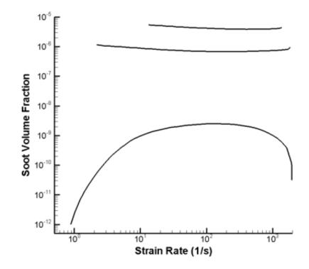
Figure 5.3: Stoichiometric value of the soot volume fraction  $f_{v,st}$  versus strain rate  $\alpha$  (log-log plot). Three solid lines: sooting and radiating flames with  $Y_{soot,R} = 0$  (bottom), 1% (middle), 5% (top).
