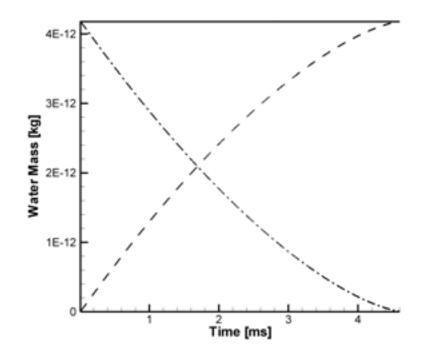
Figure C.5: Conservation of water mass in the system (droplet diameter  $20\mu$ m). The solid black curve is the total water mass in the system, expressed as the sum of the liquid water mass (dashed-dotted lines) and the gas phase water mass (dashed). The total water mass in the system remains nearly constant over the course of the droplet's lifetime (4.5 ms).
