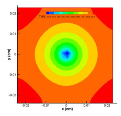
Figure C.8: Temperature isocontours for case with droplet diameter 20  $\mu$ m. The influence of the droplet spreads radially from the droplet location at the center of the domain.
