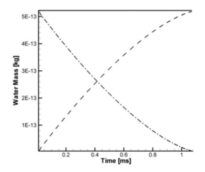
Figure C.1: Conservation of water mass in the system (droplet diameter  $10\mu$ m). The solid black curve is the total water mass in the system, expressed as the sum of the liquid water mass (dashed-dotted lines) and the gas phase water mass (dashed). The total water mass in the system remains nearly constant over the course of the droplet's lifetime (1 ms).
