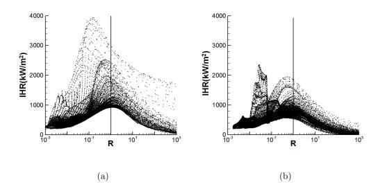
Figure 7.9: Integrated heat release rate  $(kW/m^2)$  versus weakness factor along the stoichiometric mixture fraction lines for cumulative data over the simulation time; (a) turbulent flames without spray (b) turbulent flames with spray. The vertical line denotes the R = 1 condition.
