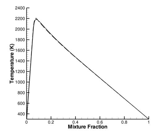
Figure B.1: Comparison between AEA and DNS flame temperatures, with  $\chi_{st} = 6 \text{ s}^{-1}$ , and the matching condition for the mixture fraction  $Z_{st,+} = 0.15$ . Solid lines denote DNS data, while dashed lines denote AEA data.
