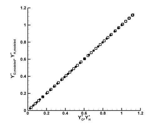
Figure A.3: DNS test of the spray-modified coupling relations presented in Equation (A.6): scatter plot showing (squares) and (solid circles) calculated from the RHS of Equation (A.21) versus the same quantities calculated as normalized hydrogen and oxygen element mass fractions.
