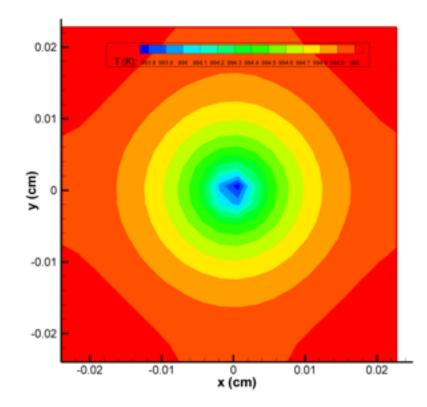
Figure C.4: Temperature isocontours for case with droplet diameter 10  $\mu$ m. The influence of the droplet spreads radially from the droplet location at the center of the domain.
