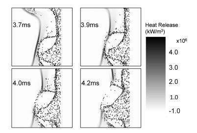
Figure 7.7: Temporal evolution of heat release rate isocontours for turbulent flame simulation with spray. The pictures correspond to the same region as those of Figure 7.5
