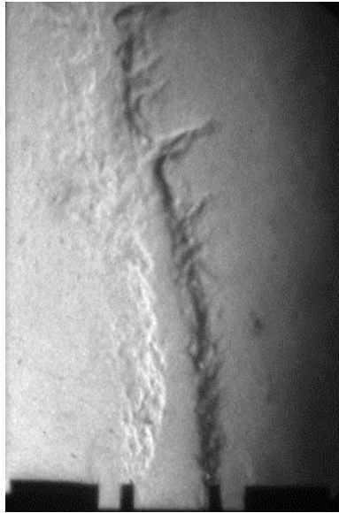
Figure 4.6: Schlieren image of H 2 -O 2 flow at u= 27/9/27 m/s and forcing at 885Hz and 60vpp
