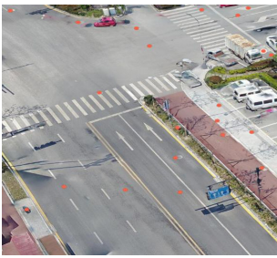
图3 井盖的二维检测结果(电子版为彩图) Fig. 3 2D detection result of manhole covers
