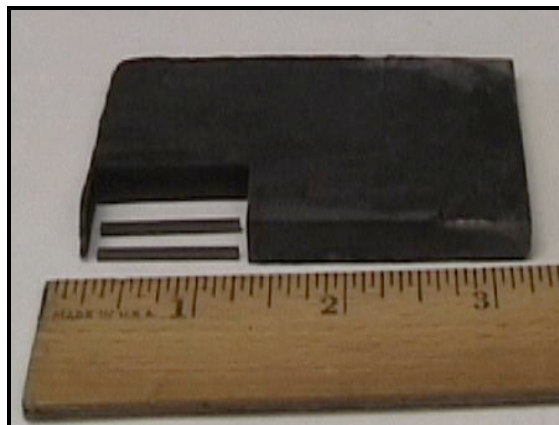
Figure 63: P2C consolidated Ti-48%Al-2%Nb-2%Cr samples of dimensions 3 inches x 2.25 inches x 0.25 inches with bend bars machined for four-point bending tests
