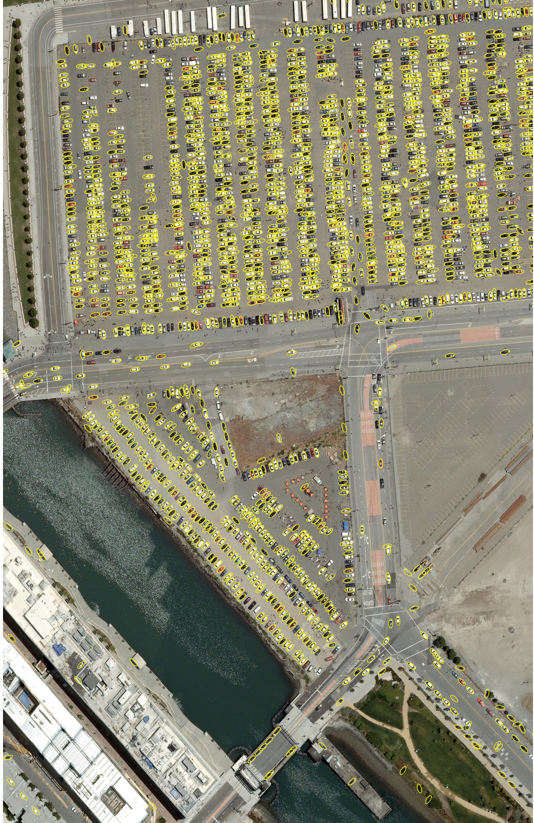
Figure 3.22: Performance of our vehicle detector on a large panoramic image overlooking the parking lot of the San Francisco Giants stadium. © 2009 Google
