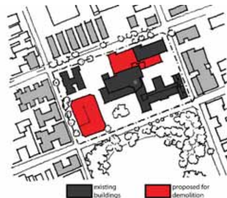
Figure 70 - Schematic Site Demolition proposing the salvage of most of the existing hospital buildings with the exception of the parking garage and emergency department buildings
