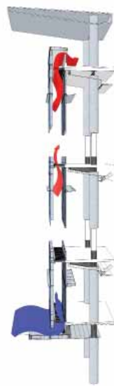
Figure 56 - Thermal buffer concept based on Author's analysis of double-glass facade on the Seattle Justice Center by NBBJ Architects
