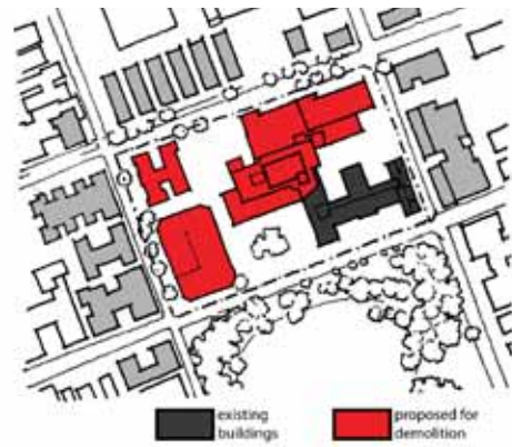
Figure 68 - Schematic Site Demolition proposing demolition of all buildings on the site with the exception of the two earliest hospital buildings
