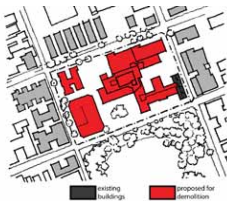
Figure 67 - Schematic Site Demolition proposing demolition of all buildings except original hospital building
