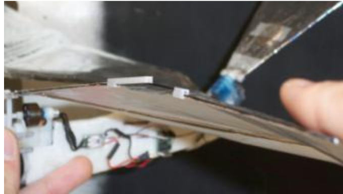
Figure 18: Wings with one-way compliance
