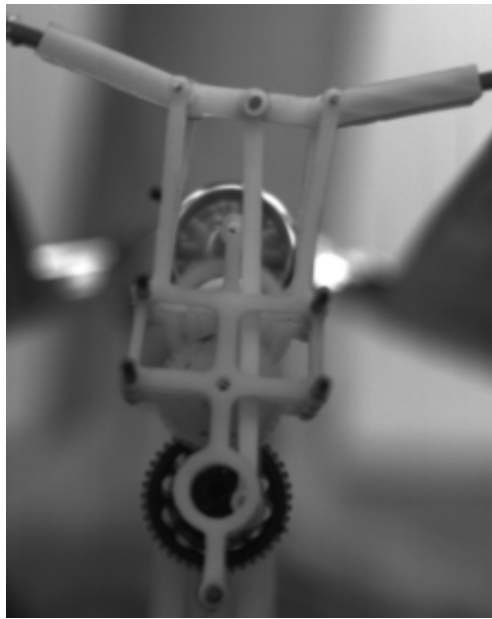
Figure 62: Asymmetric deflection of the flexural frame
