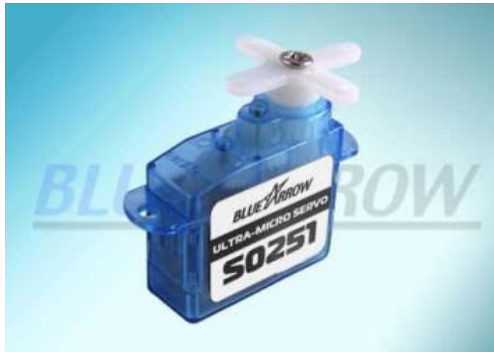
Figure 52: Blue Arrow S0251 servo used for tail rudder actuation [51]
