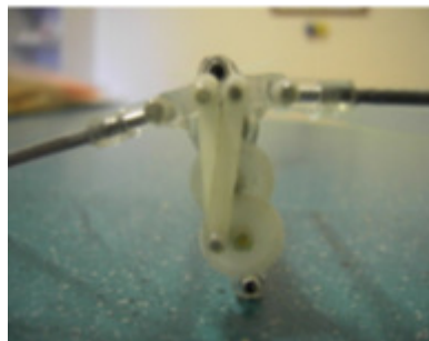
Figure 21: Chung Hua University MAV double pushrod mechanism [31]
