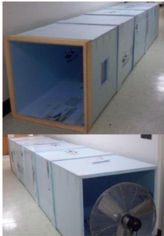
Figure 37: Tunnel used for lift testing of the MAV
