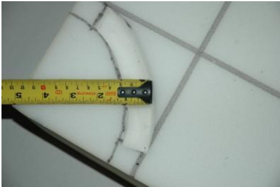
Figure 4.4: Arc Groove in the Polyurethane Foam.
