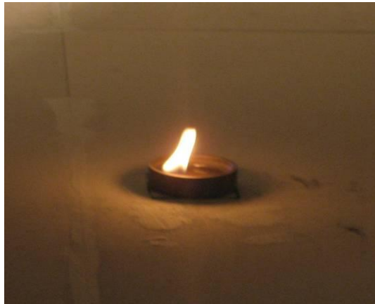
Figure 5.4: Flamelet Due to Unevenly Spread Heptane.
