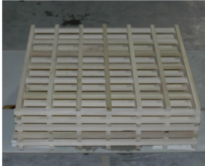
Figure 4.3: A Wood Crib Before Testing.
