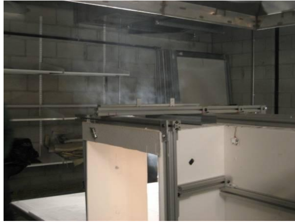
Figure 5.2: Smoke Exiting the Scaled Corridor.
