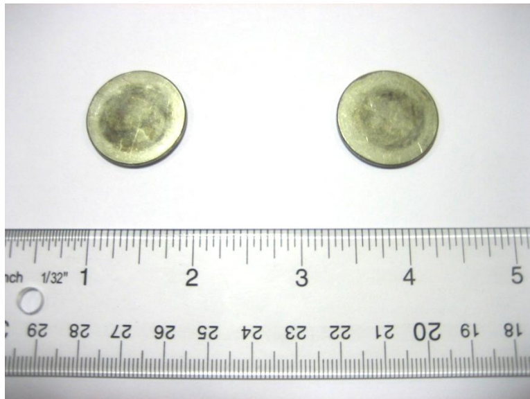
FIGURE 3-1. Photograph of Membrane I (left) and Membrane II (right) before pressure testing.
