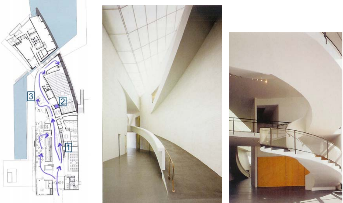
Figure 4.xx Ground floor circulation diagram depicting three means of circulating: (1) the ramp system, (2) the elevator, and (3) the asymmetrical spiral stair. (Author)
