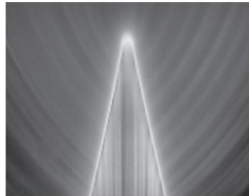
Figure 1.17 Deviation of streamlines through an inclined flame (left).
