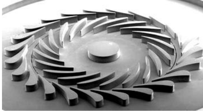
Figure 1.1 Schematic of the MIT micro-gas-turbine engine showing the radial compressor/turbine unit, combustion chamber and the electrical generator incorporated in the compressor. A photograph of the MEMS fabricated turbine blades is also shown [3]
