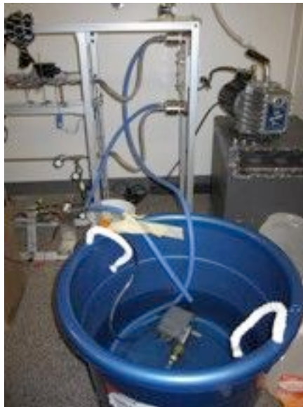
Figure 16: External Water-Cooled Condenser for the two-Phase Microgap Channel Apparatus.
