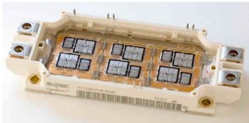
Figure 8: High Power IGBT Module [7].
