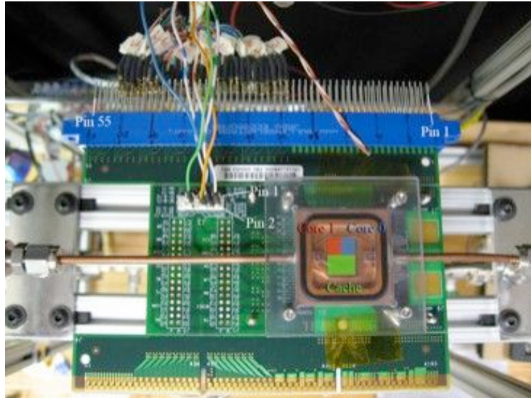
Figure 22: Assembled Intel TTV Showing Locations of the Three Heater Zones.
