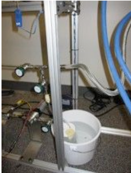
Figure 17: Pressure Relief Reservoir for the two-Phase Microgap Channel Apparatus.
