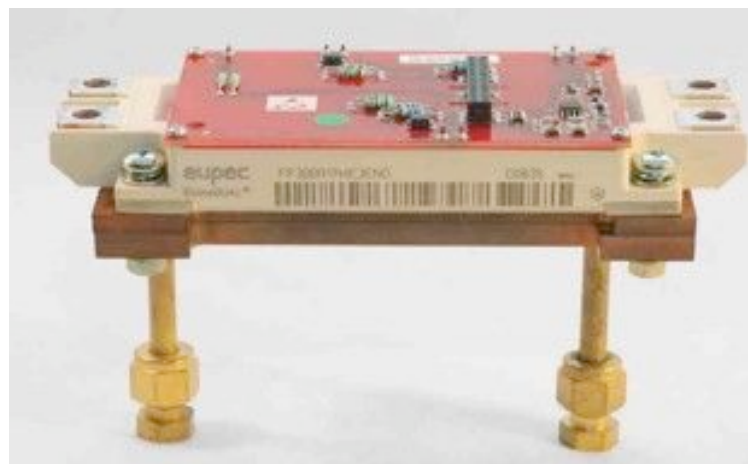
Figure 8: High Power IGBT Module [7].
