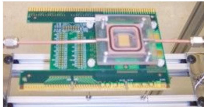
Figure 25: Hermetically Sealed Microgap Channel.
