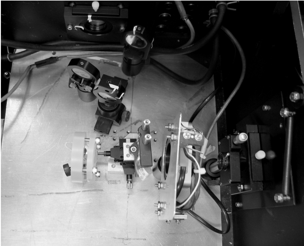
Picture of the cell used for solid/liquid interface study. The cell is made of Kel-F:
