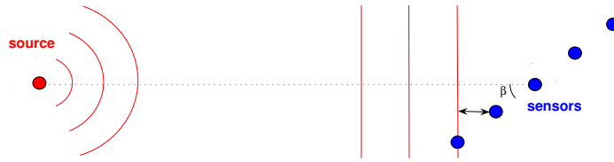
(a) uniform linear array
