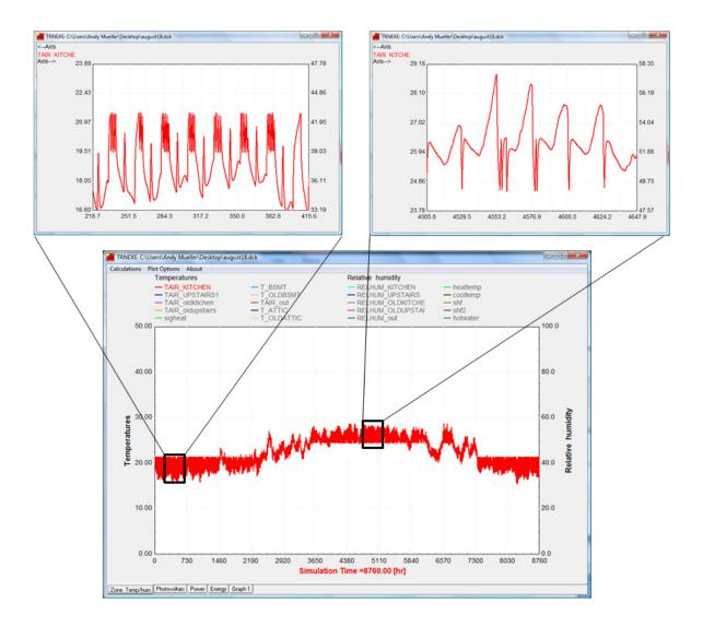
Figure 20: Low- Energy House Temperature Readings
