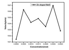
Figure 5. The acoustic velocity depends on particle concentration
