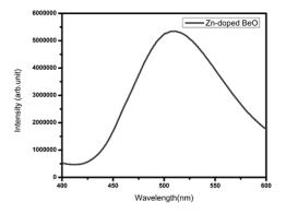
Figure 4. The photoluminescence peak of Zn doped BeO nano particles
