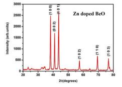
Figure 1. XRD pattern of Zn-doped BeO nanoparticles calcined at 840°C
