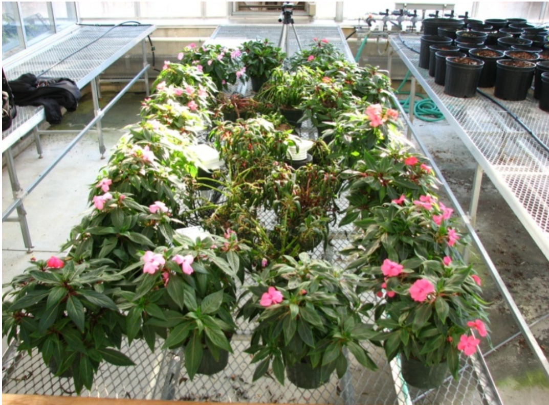
Figure 3.5. Greenhouse experimental setup with 32 ‘New Guinea’ impatiens planted in 15cm diameter x 10.5cm high containers. Four repetitions of each sensor (ECH 2 0-TE and 5TE) were randomly assigned to different containers inside the experimental area with the remaining plants as guard rows
