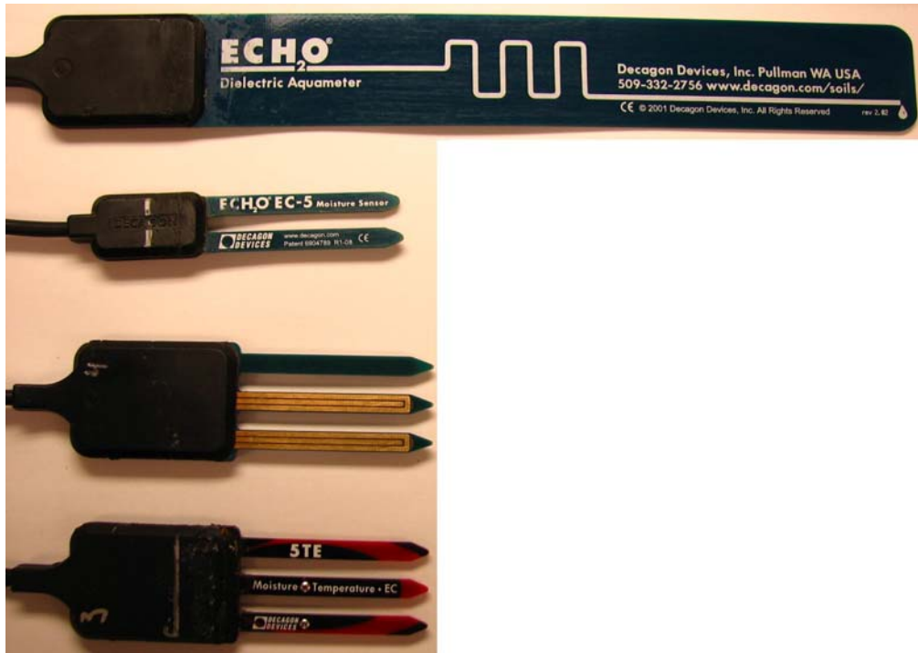
Figure 1.5. Decagon family sensors utilized in the present study. From top to bottom EC-20, EC-5, ECH 2 O-TE, and 5TE.
