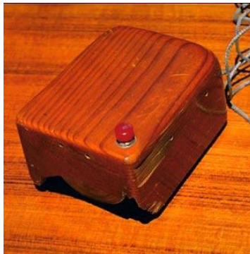
Figure 1: Douglas Englebart's original mouse design 40
