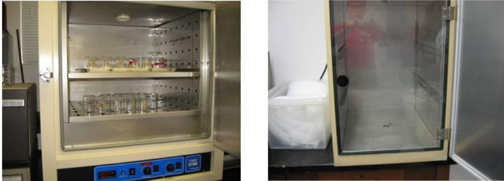
Figure 11: Oven for baking soda lime at 100°C (left); Incubator at 35°C (right)
