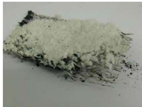
Figure 7-2. Photograph of the Carpet Material After the Cone Calorimetry Test
