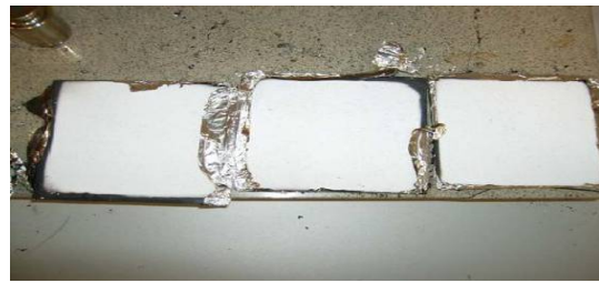
Figure 7-16. Photograph of the Wall Material After the Cone Calorimetry Test
