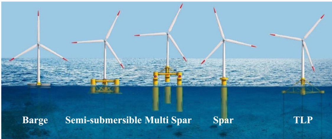
Figure 1.1 Types of floating wind foundations (Froese, 2019).
