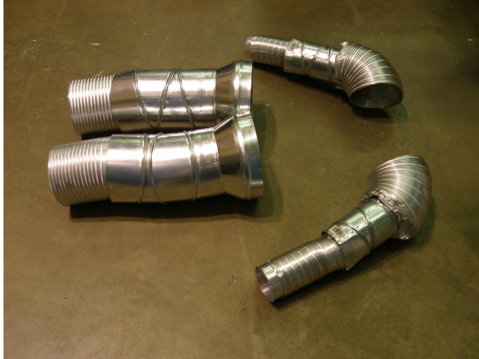
Figure 8.4: Mockups of the limbs, designed to simulate pressurized soft goods
