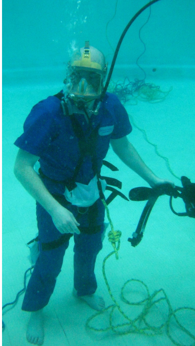
Figure 8.6: A subject wearing the ballasting harness, which simulates partial gravity.
