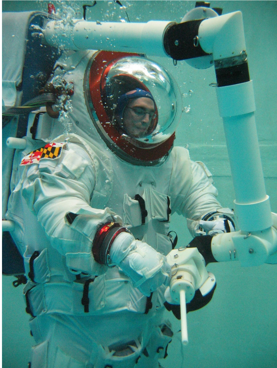
Figure 3.3: The MX-2 with a mockup of a suit-integrated robotic arm
