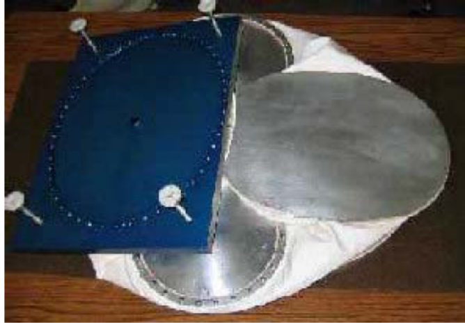
Figure 9.1: Stowed rear-entry MUT. Additional soft goods allow rings to fold flat suit architecture design could enable future planetary extravehicular activity, while minimizing costs. The analytical and experimental models developed in this work are a major step in that direction.
