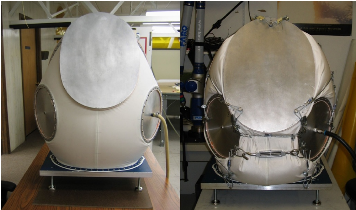
Figure 6.9: Full scale MUT model in expanded state (left) and reconfigured to nominal configuration (right)
