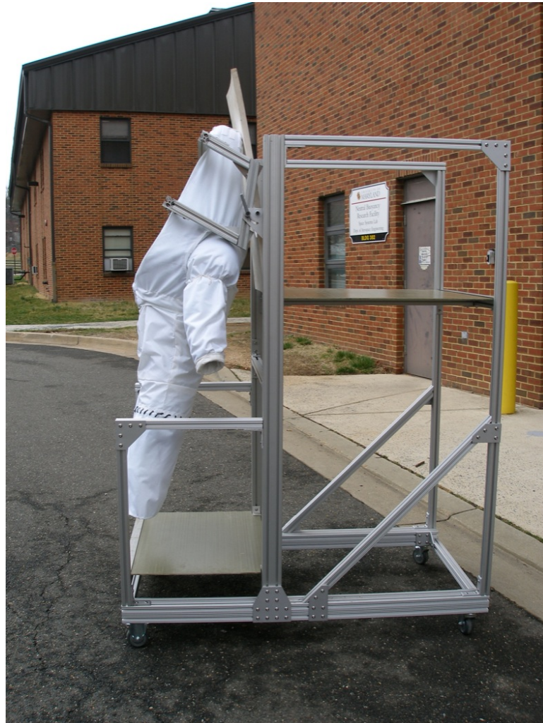
Figure 8.5: The neck-entry suit mockup hanging from the donning stand, in its nominal configuration
