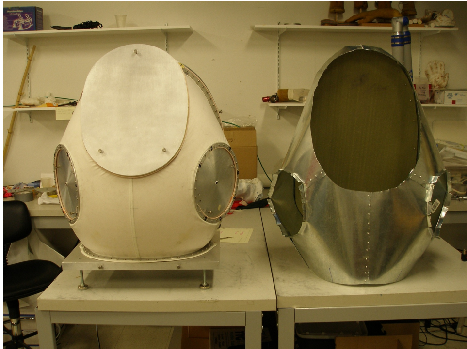
Figure 8.3: Comparison of the pressurized and expanded Morphing Upper Torso on the left, and the geometric replica on the right.
