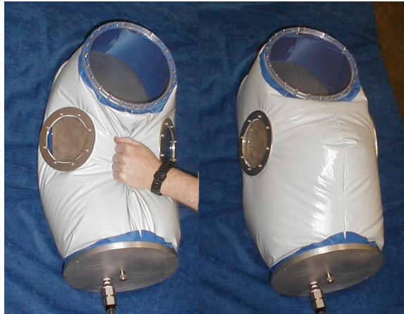
Figure 6.3: Conceptual demonstration of scye pose reconfiguration with the half-scale model
