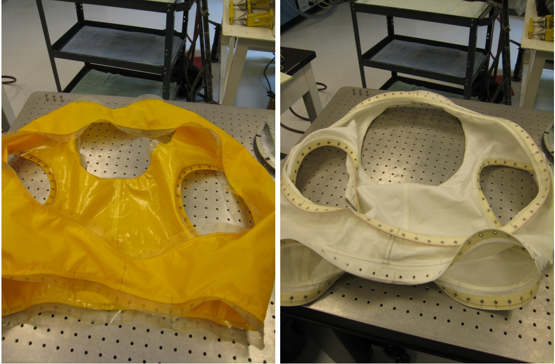
Figure 6.8: Pressure bladder and restraint layer for the full scale MUT
