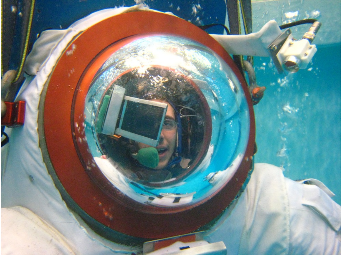
Figure A.2: During the dive pictured above, the subject uses an in-suit LCD with the backlight removed as the heads-up display. The subject brings different checklists onto the display using voice. An external helmet video camera is shown in the upper right.
