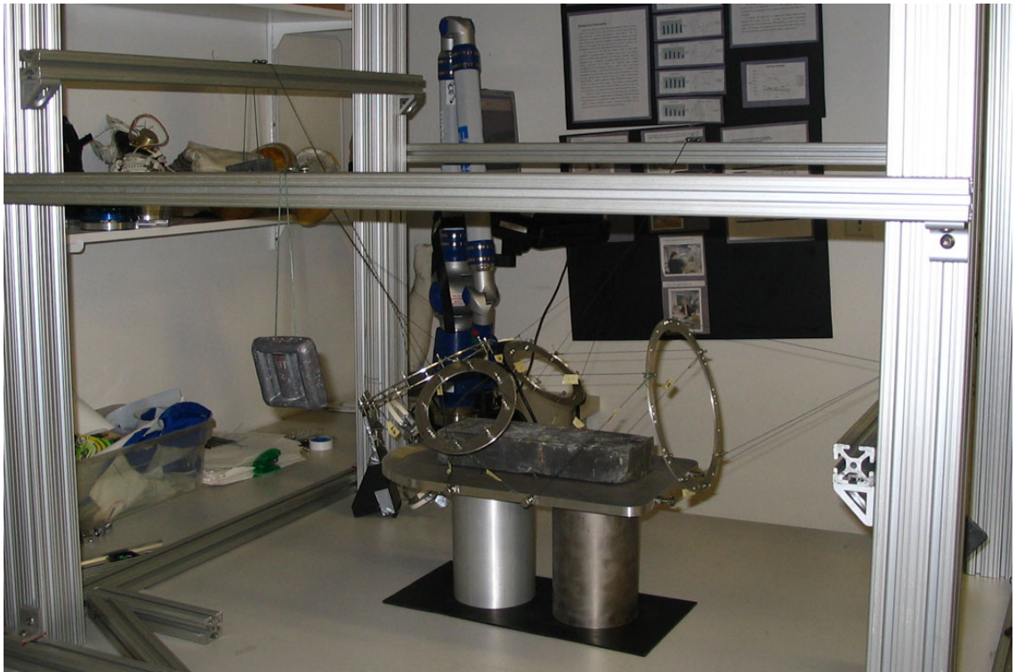
Figure 6.6: Experimental model for the isolation of pressurized fabric effects
