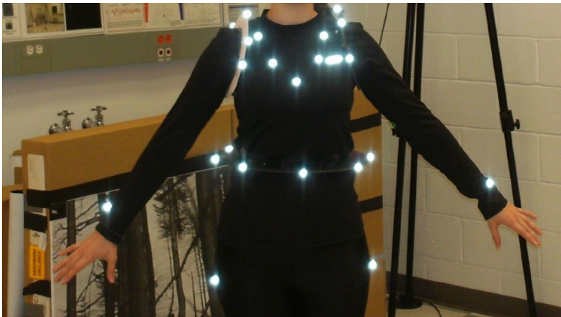
Figure 6.16: Arrangement of retro-reflective markers on test subject
