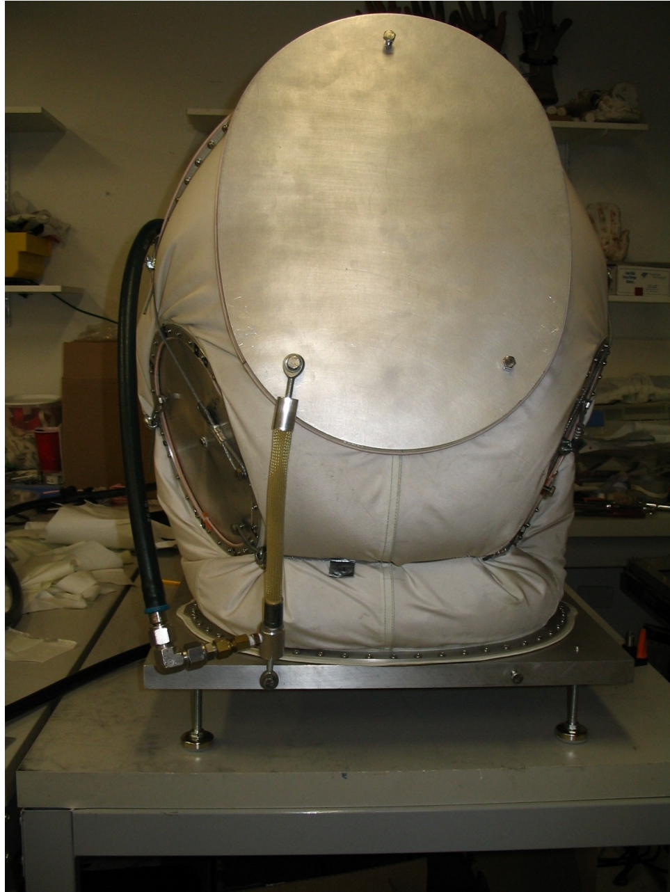
Figure 6.13: The first iteration PAM connecting the helmet ring to the waist ring
