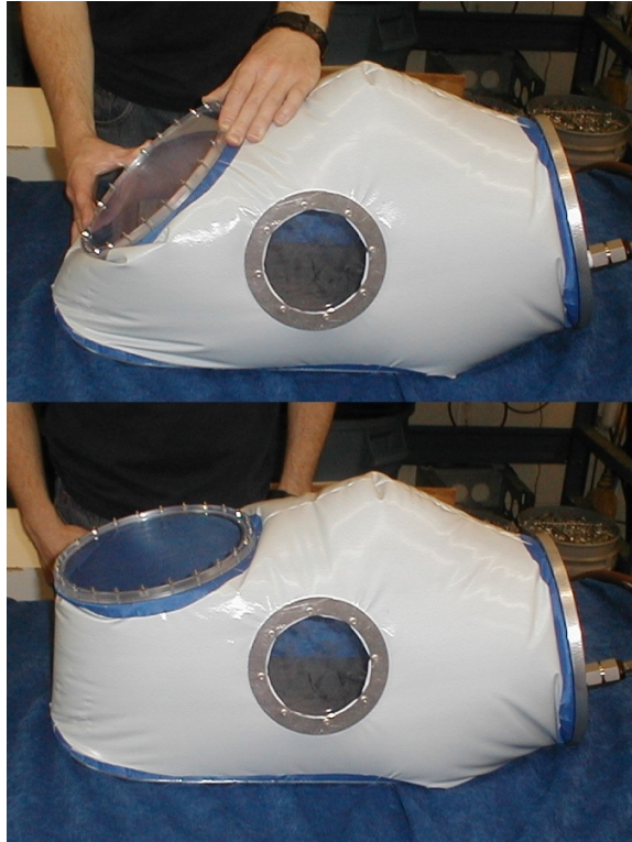
Figure 6.1: Conceptual demonstration of helmet pose reconfiguration with the half-scale model
