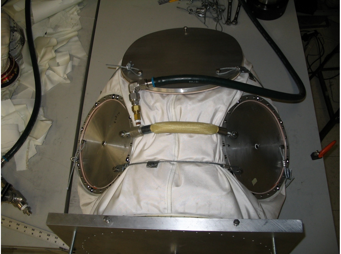
Figure 6.12: The first iteration PAM connected across the scye rings
