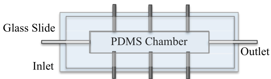
Figure 2.3 Scheme of the PDMS deposition chamber for observation of film growth (top view)
