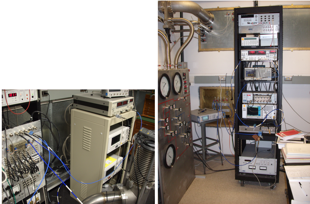
Figure 4.3: (Left) Photograph inside shielded room showing power supply rack on left and rack containing RF sources and lock-in on right. (Right) Photograph in control room. Fridge valve panel is on left. Spectrum analyzer is in lower middle of rack on right.
