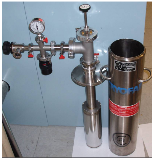
Figure 4.16: Filter cavity for suppressing phase noise. a) Design. b) Transmission of filter cavity tuned to maximum and minimum frequencies, measured at 77 K. Q ranges from 35373 to 41826. Sharp “dip” to the right of each peak is due to fortuitous interference with adjacent mode of cavity. c) Cavity and mounting brackets with quartz tuning rod. d) Assembled probe ready for cooling to 77 K.
