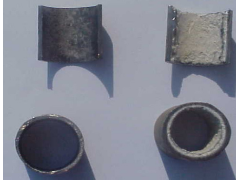
Figure 2: Seawater scaling on titanium tubes
