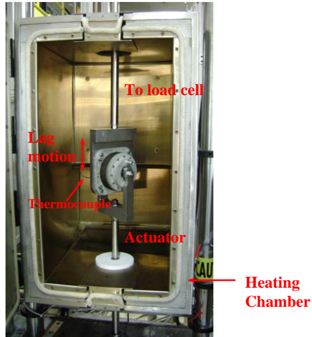
(a) FE lag damper test set-up on MTS testing machine
