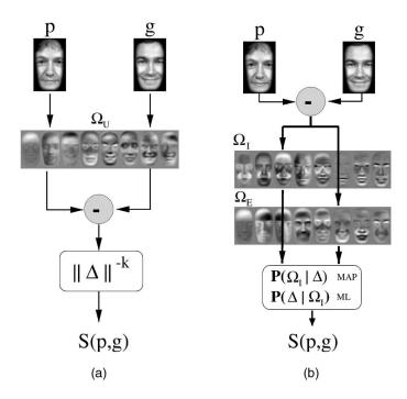
Figure 2.8: Signal flow diagrams for computing similarity **g** between two images: (a) Eigenface similarity and (b) Probabilistic similarity. The difference mage is projected through both sets of (intra/extra) eigenfaces in order to obtain the two likelihoods [52].
