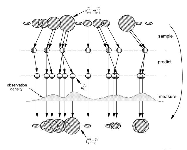
Figure 4.2: Condensation Steps. One time-step in the Condensation algorithm [34].
