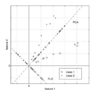
Figure 2.1: A comparison of principal component analysis (PCA) and Fisher's linear discriminant (FLD) for a two class problem where data for each class lies near a linear subspace [3].
