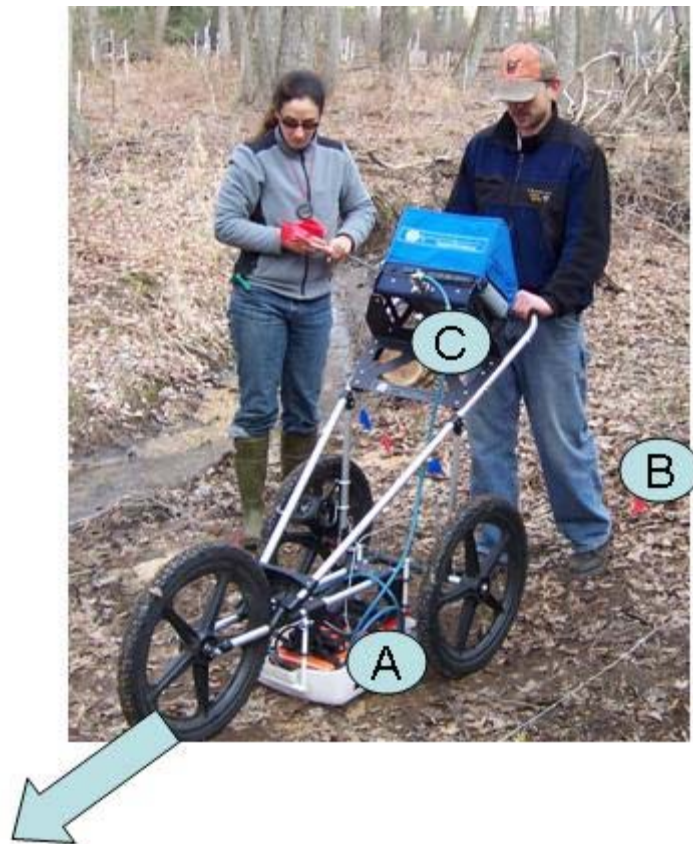
Figure 16. GPR data collection equipment. The arrow indicates the scanning direction. A = the GPR antenna housed in an orange casing within the white plastic tub; B = B-scan starting point; and C = GPR control unit and computer.
